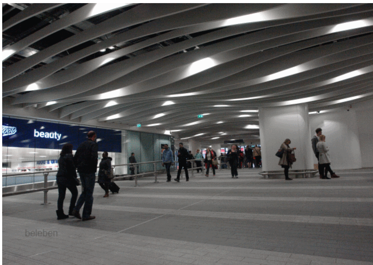
Floor patterning that could be mistaken for steps- BS 8300-2009
